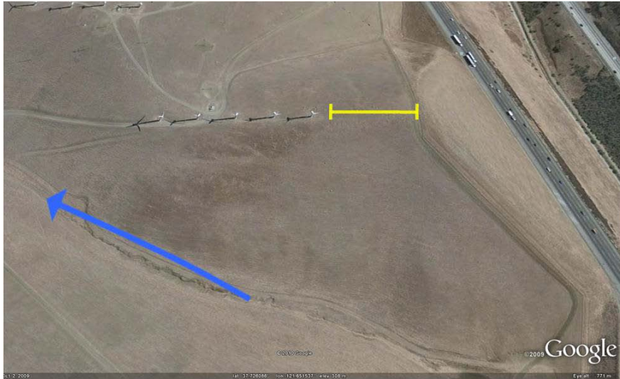
Photo 7. Turbine relocations would be relatively safer where they are set back (see yellow bar) from steep slopes facing prevailing wind directions (blue arrow).
