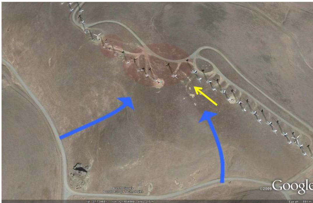
Photo 24. Wind turbines can be more hazardous where turbine rows zig-zag in direction (yellow arrow), especially where slope-accelerated winds (blue arrows) intersect the change in direction of the turbine row.
