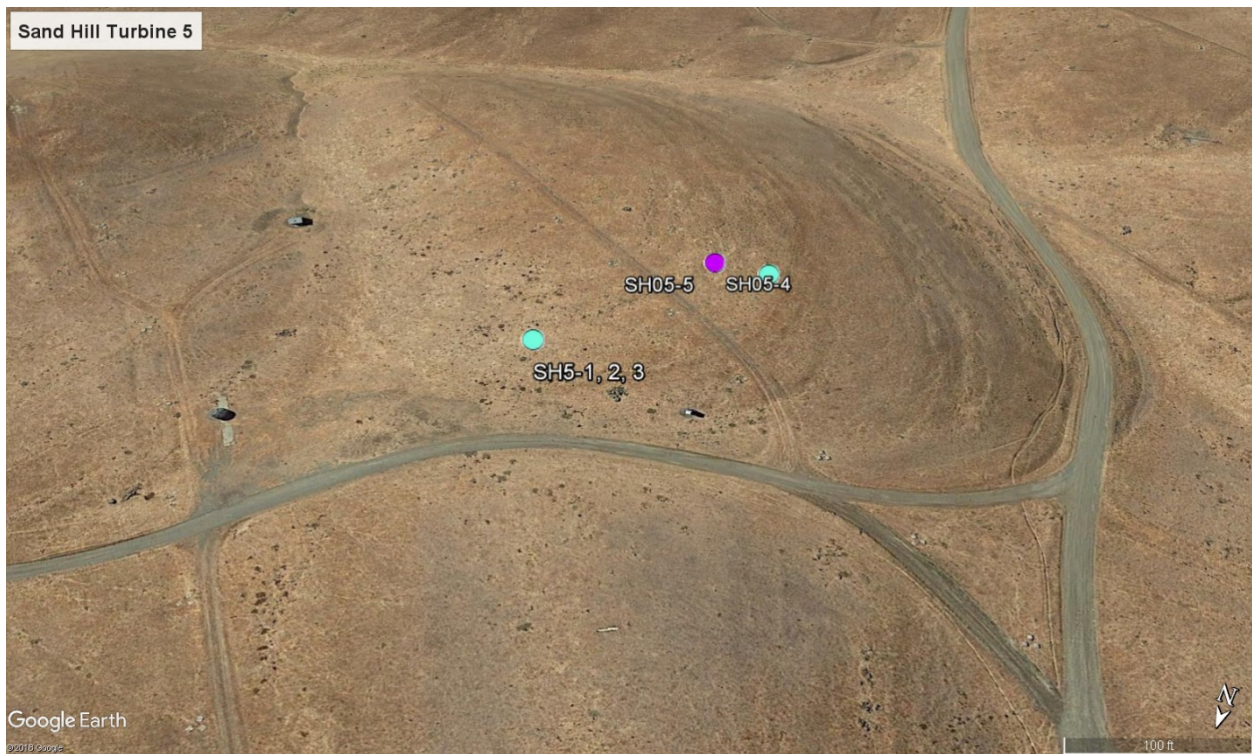
Figure 4: SH05-1,2,3 is representative of Layouts 1-3. SH05-4 was relocated 62 m SW in response to Smallwood's recommendation. SH05-5 was relocated 53 ft E in response to Estep's recommendation and is the Micro-sited Smaller Turbine Layout (Layout 5).
