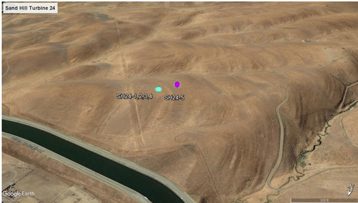
Figure 15: SH24-1,2,3,4 is representative of Layouts 1-4. SH24-5 was relocated 150 ft SW toward the hilltop in response to Estep's recommendation and is the Micro-sited Smaller Turbine Layout (Layout 5).
