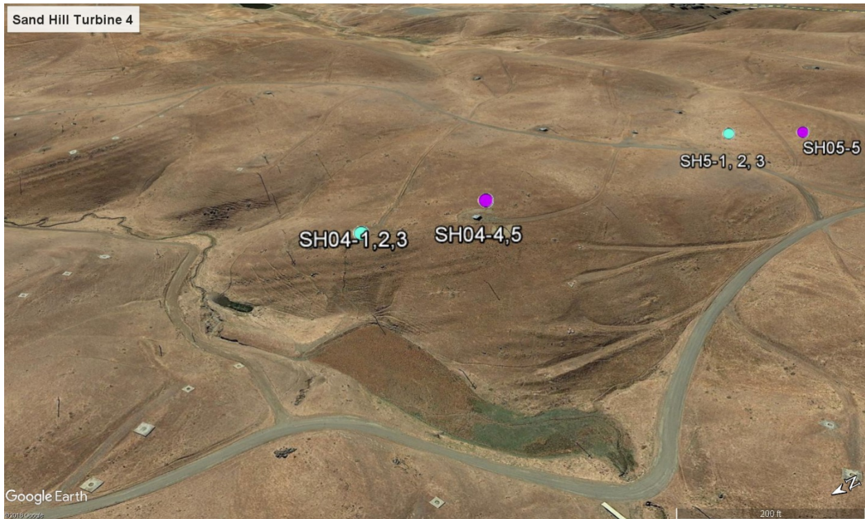
Figure 3: SH04-1,2,3 is representative of Layouts 1-3. SH-04-4,5 was relocated 80 m SW away from the ravine and closer to the top of the hill and is the Micro-sited Smaller Turbine Layout (Layout 5).
