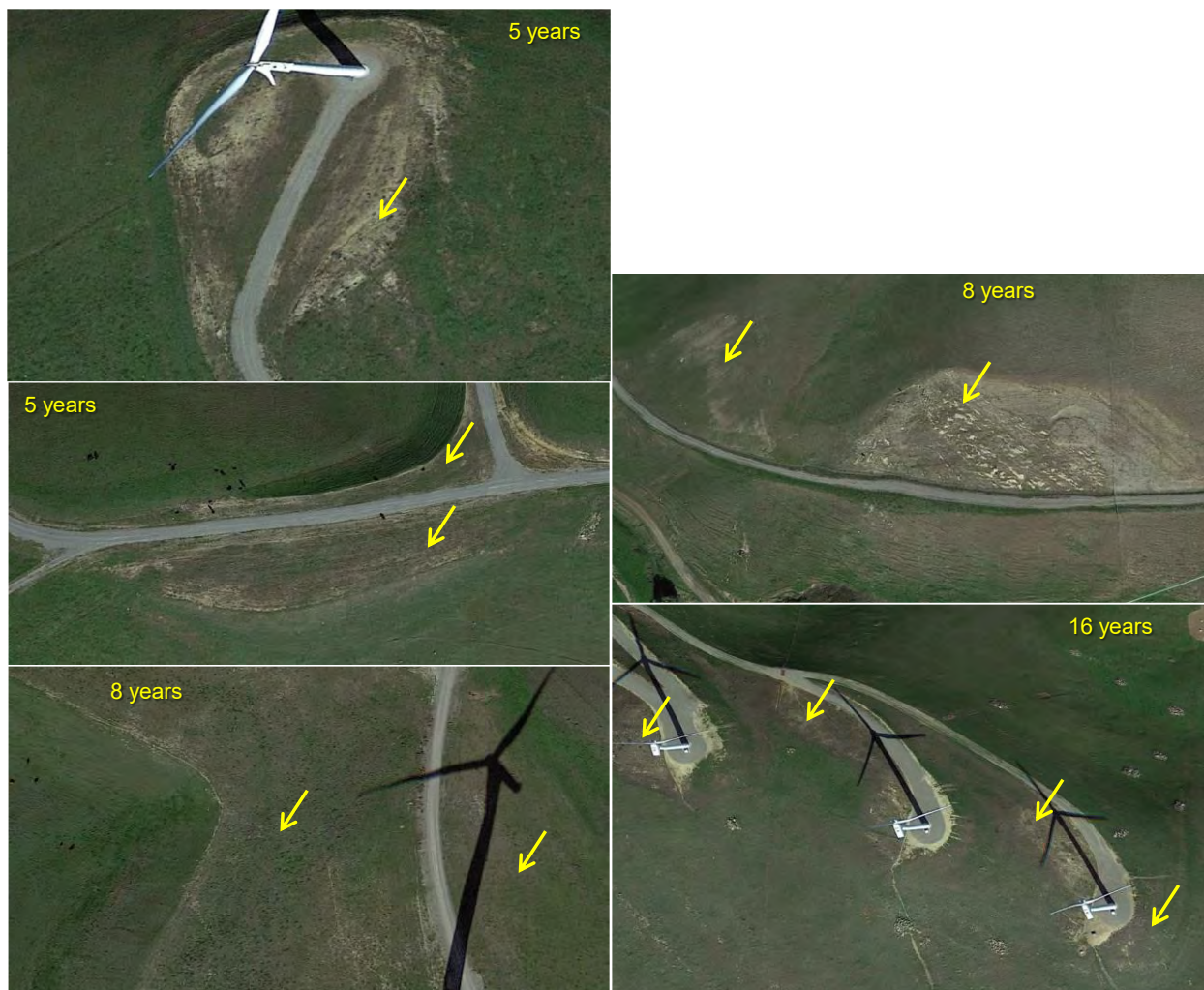
Photo 13. Effects of grading on vegetation cover in the APWRA, 5 years, 8 years, and 16 years following construction and efforts at revegetation. Yellow arrows point to some of the graded areas visible in the February 2020 Google Earth imagery, areas in which vegetation has yet to return to normal composition and density.
