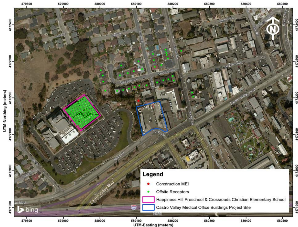
Figure 1. Project Construction Site, Point Source Locations, Locations of Off-Site Sensitive Receptors, and TAC Impacts
